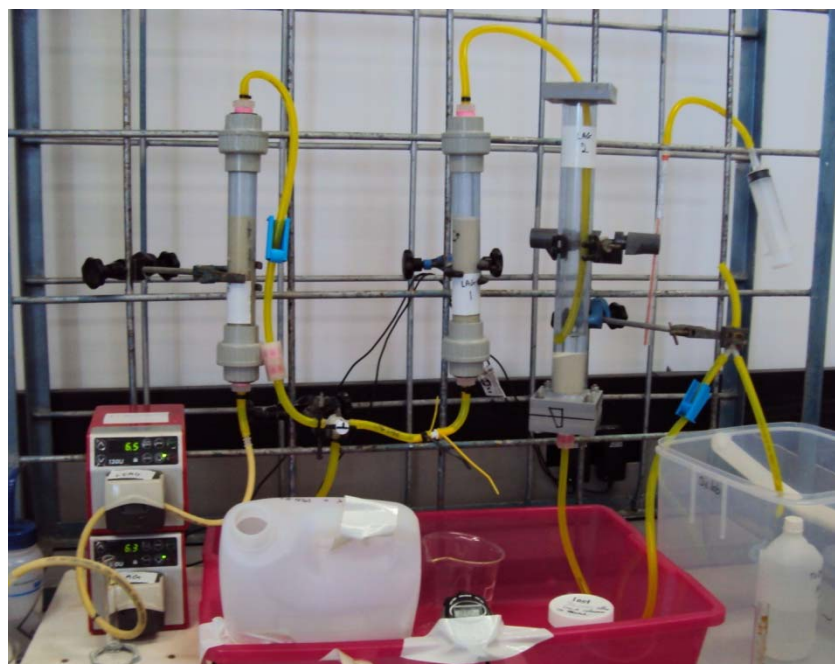
Figure 11 IX Loading Circuit Set up
