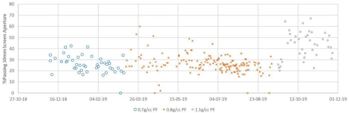
FIG 17 – Primary crusher product fines content.
