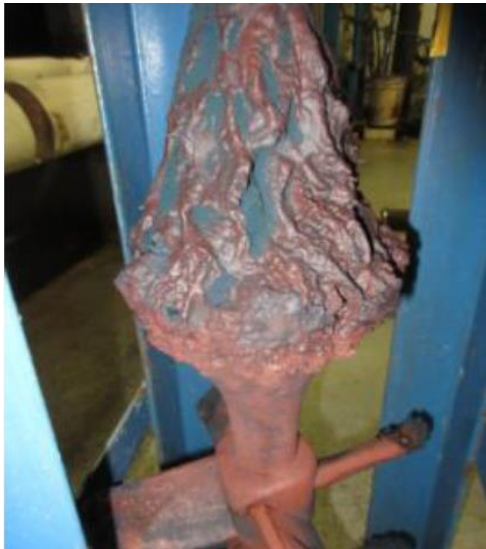
Figure 27: Metallurgical Scale on a Leach Vessel Agitator Shaft and Impeller
