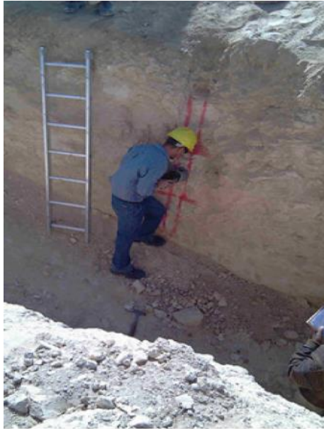
Figure 1: Radiometry mapping of trench wall (Courtesy of JUMCO)
