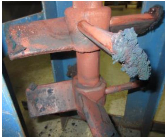
Figure 27: Metallurgical Scale on a Leach Vessel Agitator Shaft and Impeller
