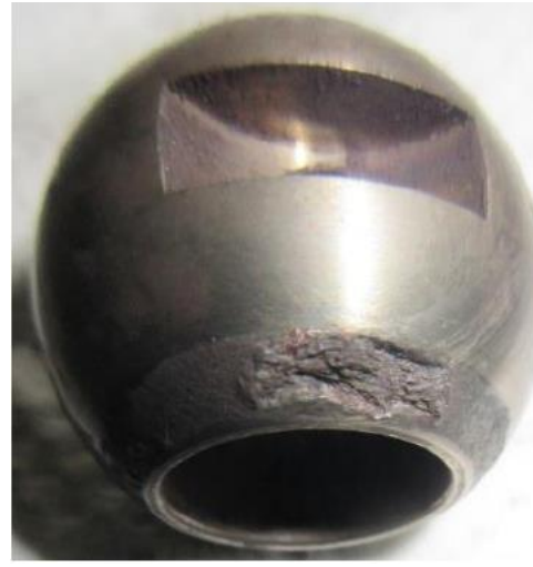
Valve Ball displaying Crevice Corrosion
