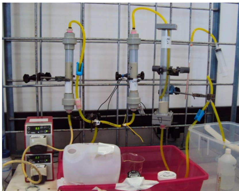
Figure 11 IX Loading Circuit Set up
